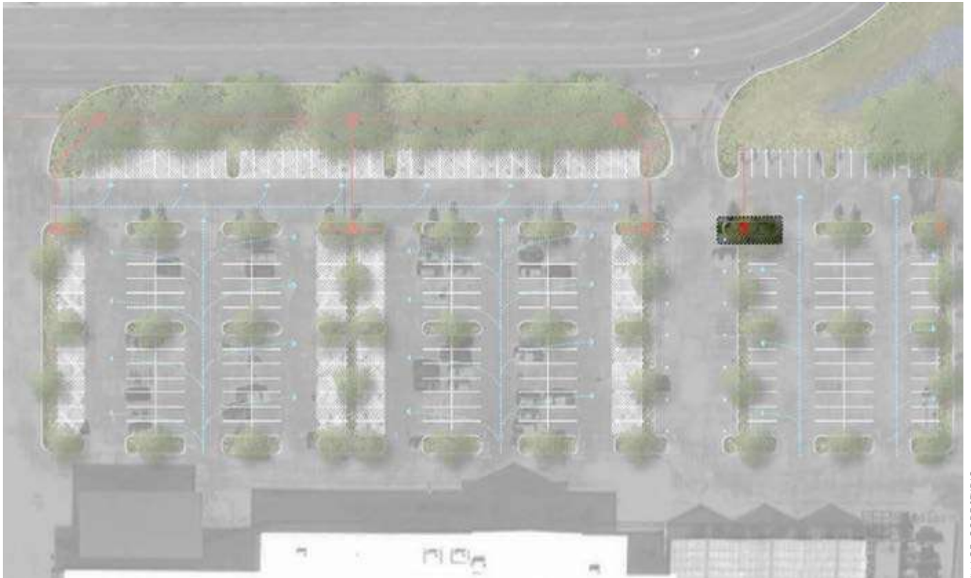
CH7-52: This image provides an example of how the required planting island might be designed and constructed to integrate the landscaping and stormwater management together.
