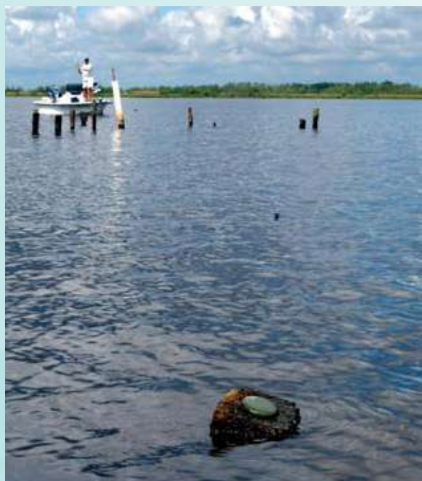
CH3-1: The USGS elevation marker in the foreground measures Louisiana's water level rise and land loss.
