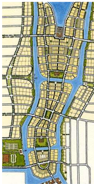
D-26 Plan view of proposed new Earth neighborhood showing canals and raised land which provide flood and stormwater protection.
