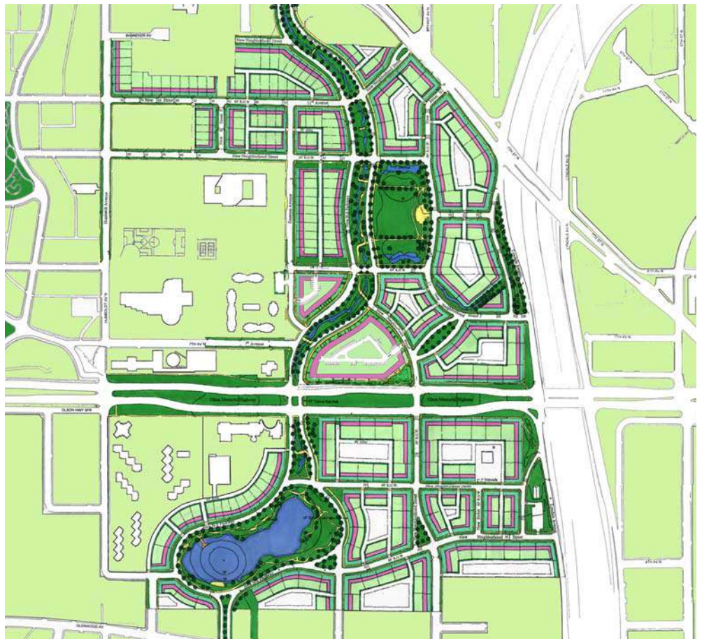
D-46 Plan showing framework of public open space and restored and reestablished natural features in the center of an urban neighborhood which had been poorly developed in a way that eliminated the natural features.
