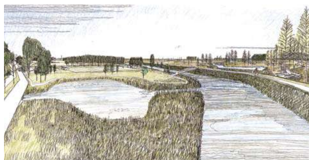
D-25 St. Bernard Parish: Proposed view of wetlands and green space along the 40 Arpent Canal and Florida Avenue demonstrates a natural alternative to concrete-lined channels as a means of water management.
