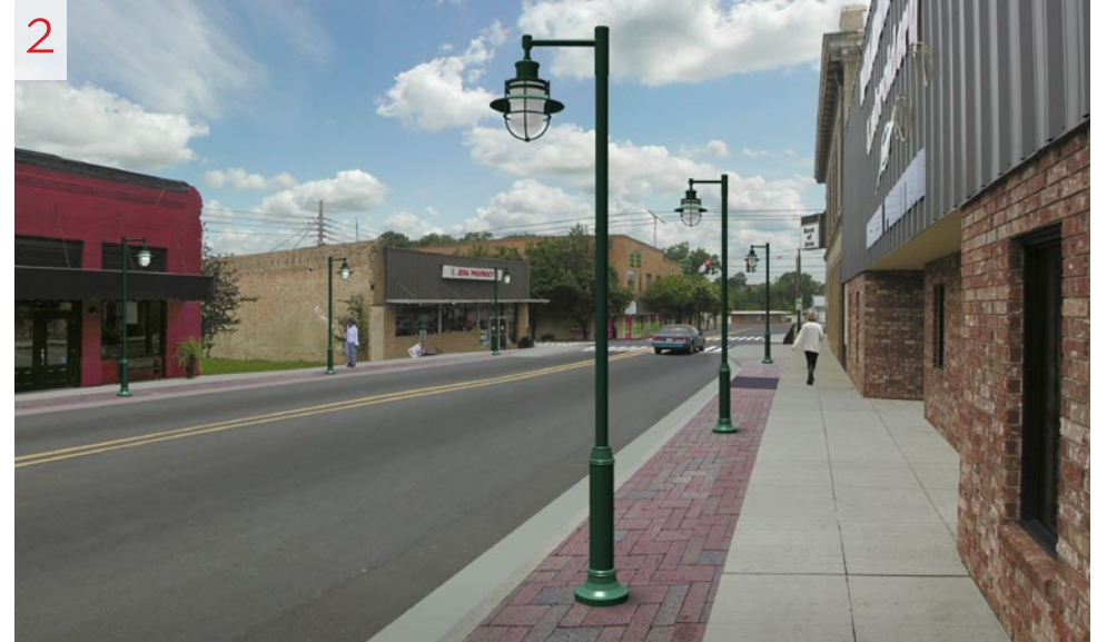
Overhead utilities moved to rear of buildings. Sidewalk width extended and pedestrian-scaled lighting installed. Striped pedestrian crossing added at intersection of Highway 84 and LA 127.
