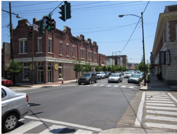
A one-way couplet system runs through downtown Hammond. Couplets are usually separated by one city block, allowing travel in opposite directions.
