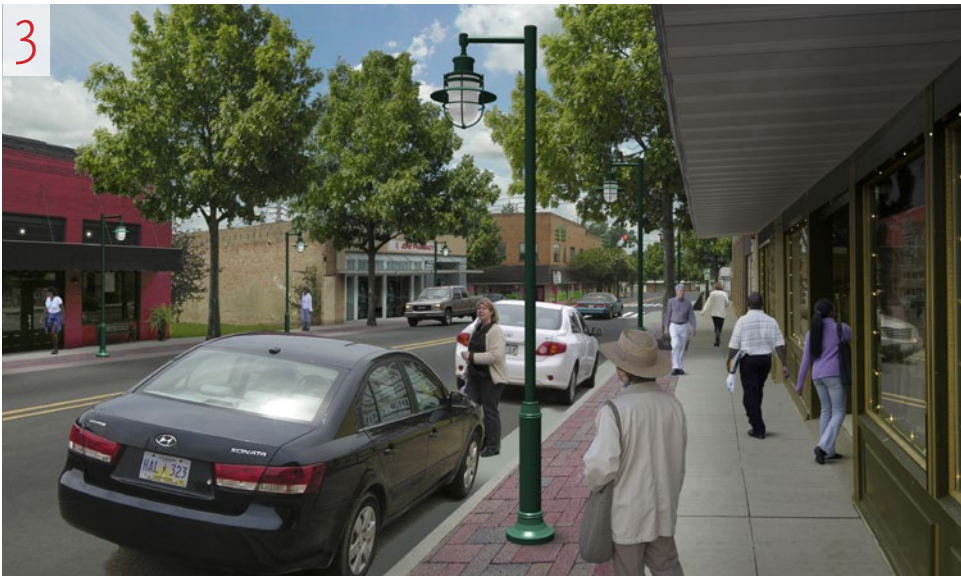
Street trees planted at regular intervals so as not to interfere with overhead canopies. Width of on-street parking lane reduced to accommodate wider sidewalk. Blank walls replaced with storefront windows that enhance the pedestrian experience.
